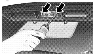
2. Rotate the socket 1/4 turn counterclockwise.
